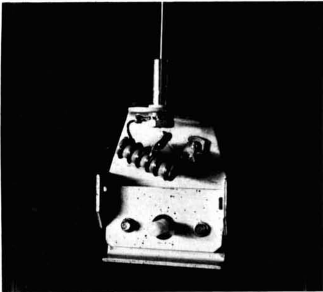
Matching coil is located under the mount to inhibit radiation.
